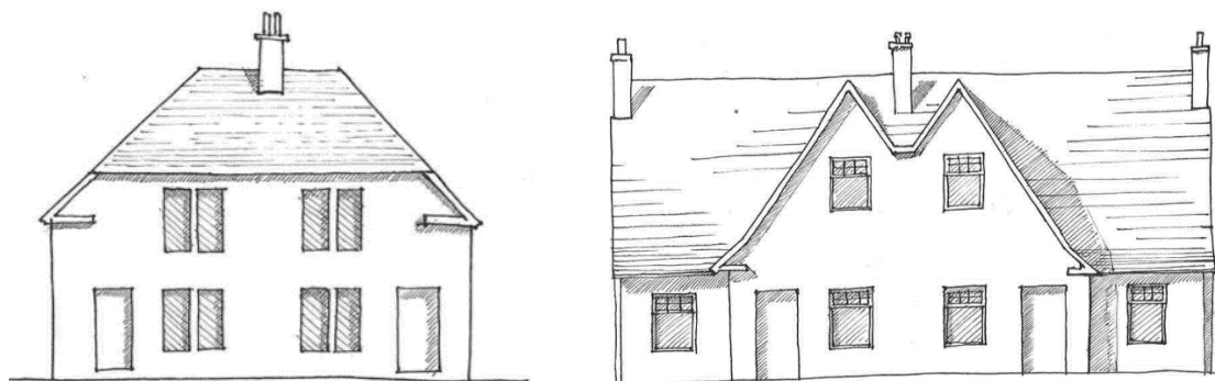
Figure 9: Jerkinhead roofs present lower eaves at the sides (left). High-pitched roofs like that of the recognisable Type-B housetype are characteristic of the Garden City (EAC DP&R).
