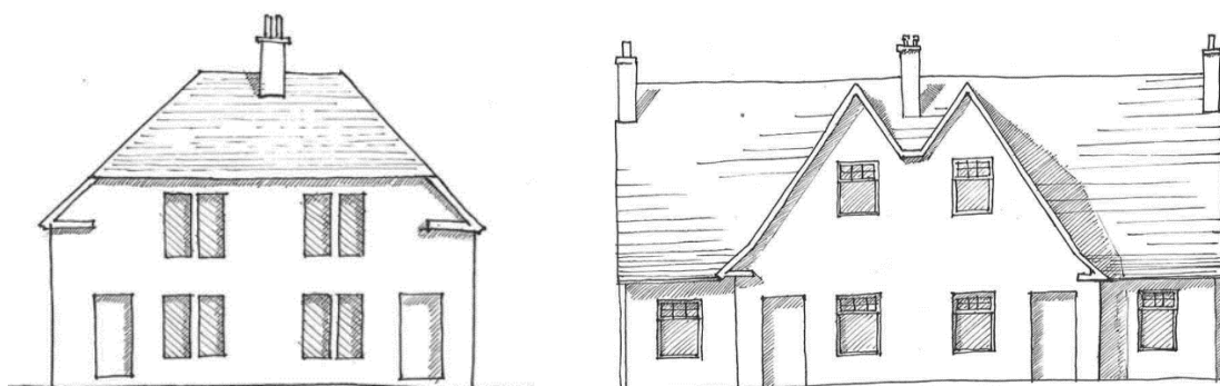
Figure 5: (left) Rectangular box with jerkinhead roof; (right) "Type B" presents 45-degree gabled roofs (EAC DP&R).
