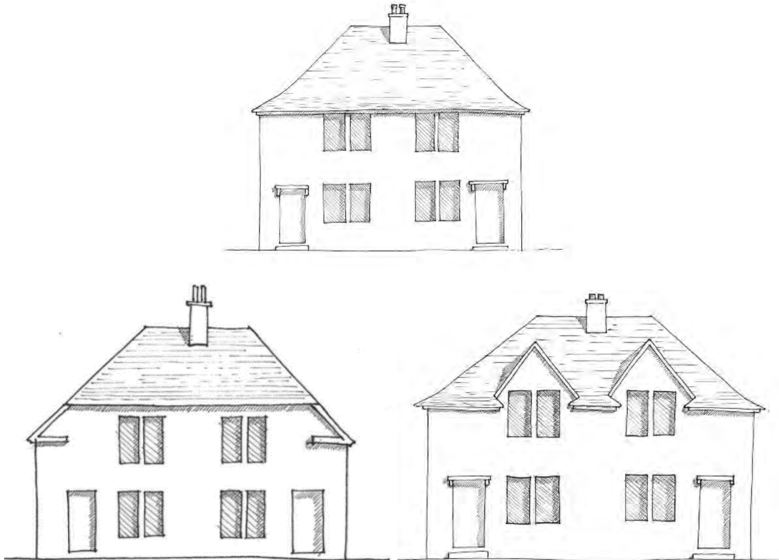
Figure 25: (top) Rectangular box semidetached house; (left) variation with jerkinhead roof; (right) variation with two street-facing gables.
