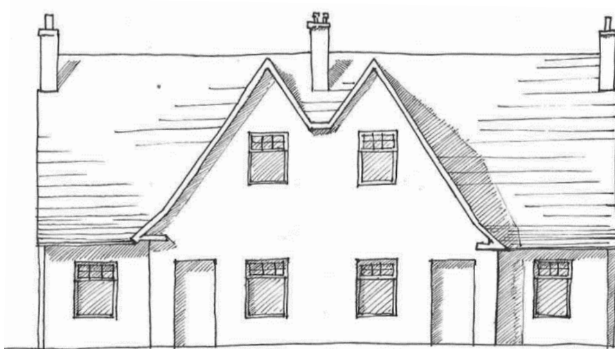
Figure 24: "Type B" presents 45-degree gabled roofs.
